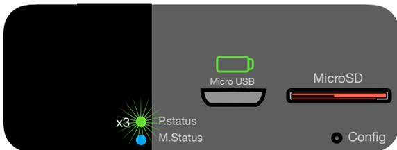
In some cases you may see the P.status LED flash three times. This is to indicate that Poly has acknowledged that a Micro SD has been inserted into the Micro SD card slot and has been recognized. If a Micro SD card is present during boot up of the Poly the P.status will flash three times. It is ok to take a Micro SD card in and out of the Poly while powered on but make sure no music is playing from the Micro SD card to avoid risk of corrupting the data..
