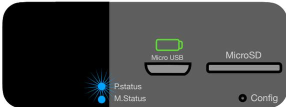
If the P.status LED is blinking blue rapidly. Poly is unable to either connect to the WiFi network just attempted in the Poly setup or to a previously connected WiFi network. In the case of a new network use the Sim Card Tool included and push the Config button for 7 seconds, Remove the Sim Card Tool and wait up to 10 seconds for Poly to enter Access Point Mode, which is indicated with P.status flashing from blue to green. You can now attempt setup again.
