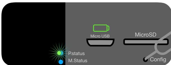
Poly can be used with more than one WiFi network for example a home WiFi network and a mobile hotspot for home and on the go use. To add an additional network use the Sim Card Tool included with the Poly to press in the Config button for 7 seconds. Remove the Sim Card Tool and wait up to 10 seconds for Poly to enter Access Point Mode which is indicated with P.status flashing from blue to green.
